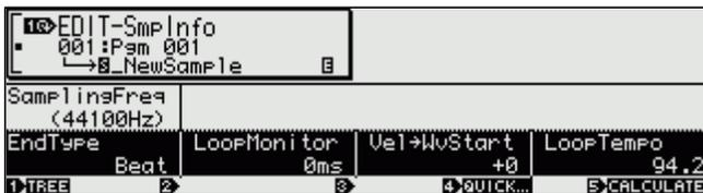
[EDIT], [TRIM/LOOP] Sample Info screen. (Use Knob 1 to see this screen). Set the End Type to BEAT. Loop Tempo can be calculated in BPM by pressing KNOB 5. The Loop Monitor parameter let's you hear just ahead of the loop start point – push and hold it to preview the data up to ½ a second (500ms) – it plays the lead in data only once. Now return to the previous screen. Your defined loop will be displayed in terms of Beats (close to
